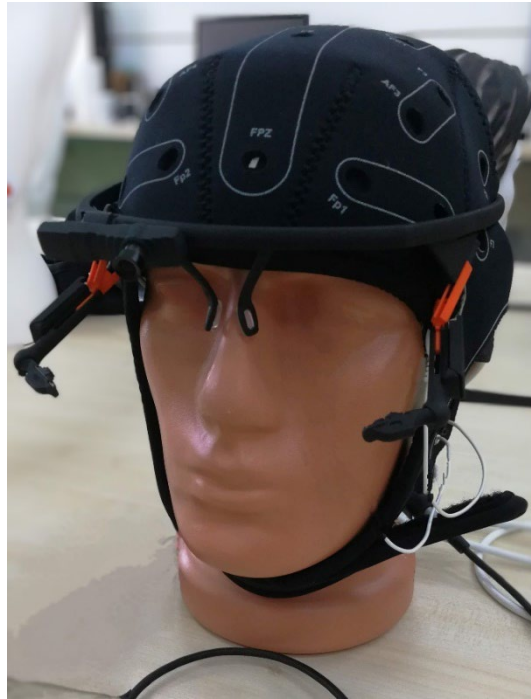
Figure 17: Neoprene EEG cap, fNIRS headband, and wearable eye tracker Pupil Labs Pupil Core worn.
