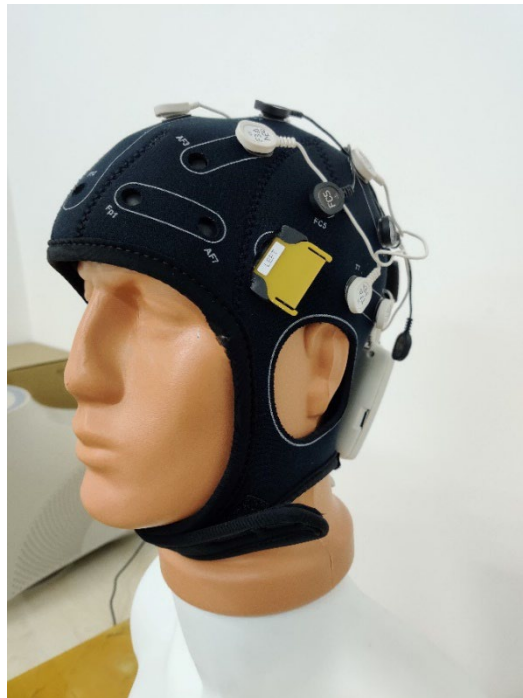
Figure 19: Neoprene EEG cap cabled with dry-electrodes and fNIR forehead band protruding from the cap through F7, F8 channels. Left-hand side view.
