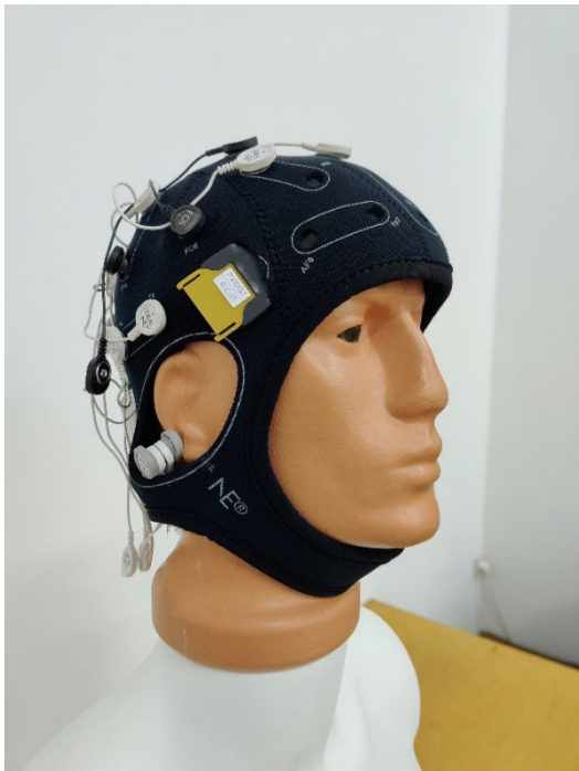
Figure 18: Neoprene EEG cap cabled with dry-electrodes and fNIR forehead band protruding from the cap through F7, F8 channels. Right-hand side view.
